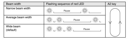
Pressing the A1 key for 2 seconds saves the selected type of beam width. The parameter assignment process is then complete and the sensor returns to normal mode. If you press the A1 briefly instead, you go back to Level 1 (parameter assignment of output function).
