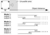
A1  $\longrightarrow \infty$ , A2  $\longrightarrow \infty$ : Object presence detection. Both outputs operate according to the selected mode, if an object is located within the detection range.
