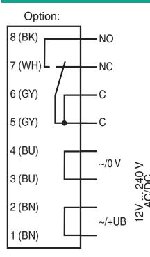
The relay-functions "NC" and "NO" bear on the switching mode "Dark-ON". This complies to the default setting of the light/dark switch (factory setting).
