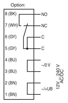
The relay-functions "NC" and "NO" bear on the switching mode "Light-ON".
