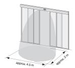
Installation height 2200 mm / angle of detection field  $30^{\circ}$ Antenna position:
