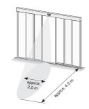
Installation height 2200 mm / angle of detection field  $30^{\circ}$ Antenna position:
