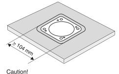
After removal of the metal screen the proximity switch can no longer be mounted as an embedded installation.
