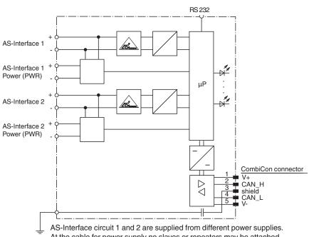
At the cable for power supply no slaves or repeaters may be attached. At the cable for AS-Interface circuit no power supplies or further masters may be attached.
