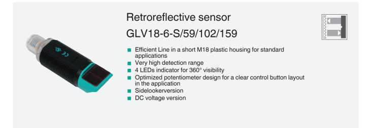
Retroreflective sensor, M18 threaded housing design, plastic housing, side optical face, 5.5 m detection range, red light, dark on, DC version, NPN output, M12 plug
