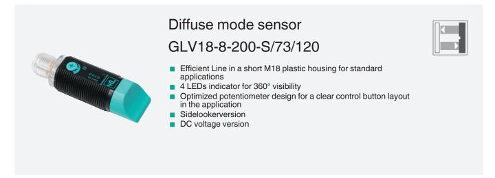
Diffuse mode sensor, M18 threaded housing design, plastic housing, side optical face, 200 mm detection range, red light, light/dark on, DC version, 2 PNP outputs, M12 plug
