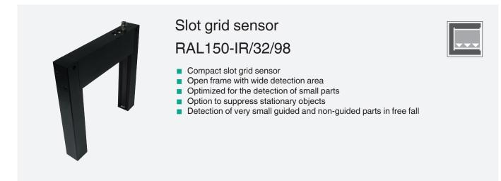
Compact slot grid sensor, optimized for detection of small parts, 150 mm slot width, infrared light, PNP output, M8 plug
