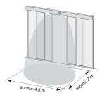
Installation height 2200 mm / angle of detection field 30° Antenna position:
