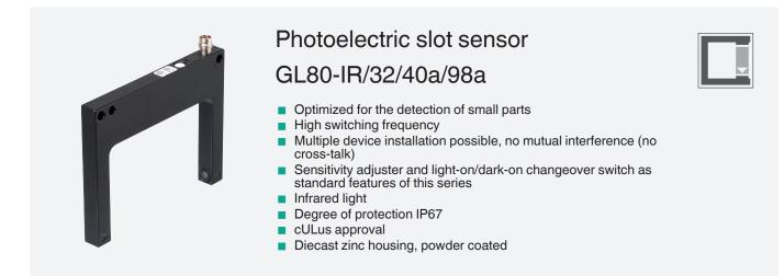
Photoelectric slot sensor, zinc pressure diecast housing, 80 mm slot width, infrared light, light/dark on, sensitivity adjuster, DC version, PNP output, 3 pin M8 plug
