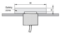
Metal objects must not be inserted or handled in the area of the safety zone during operation.
