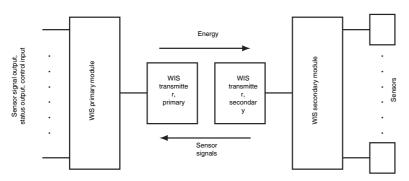
The sum of the currents of all sensors attached to the WIS secondary module must not be greater than the maximum transferable current. This is calculated by dividing the transferable power by the 12 V provided by the transmitters.
