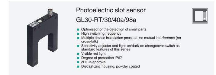
Photoelectric slot sensor, zinc pressure diecast housing, 30 mm slot width, red light, light/dark on, sensitivity adjuster, DC version, NPN output, 3-pin M8 plug
