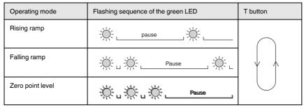
• Return the selector switch to position N when the desired operating mode is displayed.
