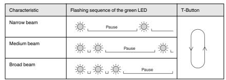
Return the selector switch to position N when the desired beam breadth is indicated.
