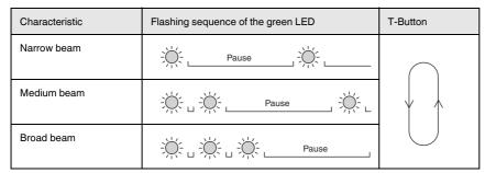
Return the selector switch to position N when the desired beam breadth is indicated. Note: Acceptance of the ultrasonic beam breadth into the permanent memory of the sensor does not take place until the
