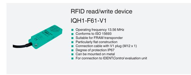
HF RFID read/write device, ISO 15693, for IDENTControl
