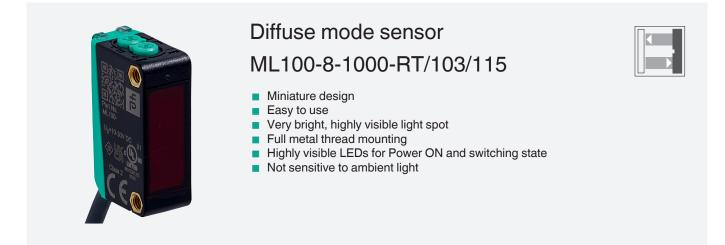
Diffuse mode sensor, plastic housing, 1000 mm adjustable detection range, red light, light/dark on, pnp output, fixed cable
