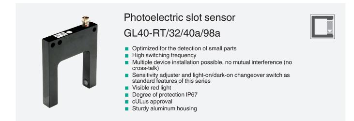
Photoelectric slot sensor, aluminum housing, 40 mm slot width, red light, light/dark on, sensitivity adjuster, DC version, PNP output, 3 pin M8 plug
