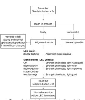
More stringent adjustment requirements: Ensure that the device is correctly aligned in the near range of 0.2 m ... 0.6 m.
