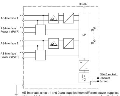
AS-Interface circuit 1 and 2 are supplied from different power supplies. At the cable for power supply no slaves or repeaters may be attached. At the cable for AS-Interface circuit no power supplies or further masters may be attached.
