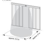
Mounting height 2200 mm / tilt angle 30° Antenna position:
