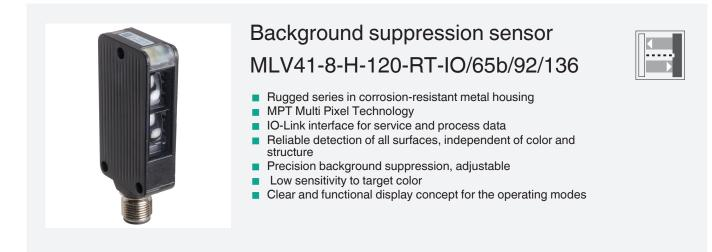
Diffuse sensor with measurement core technology, compact housing design, background suppression and 3 further adjustable operating modes, IO-Link interface, 120 mm adjustable detection range, red light, 2 push-pull outputs, M12 plug
