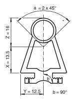
\* effective sensing angle according to EN 1760-2
