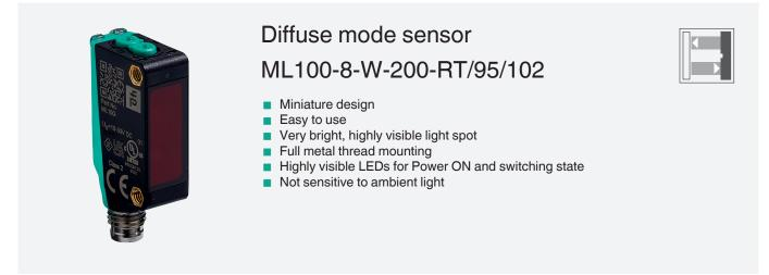
Diffuse mode sensor with rectangular light spot for clear object detection, 200 mm detection range, red light, light/dark on, sensitivity adjuster, DC version, NPN output, M8 plug
