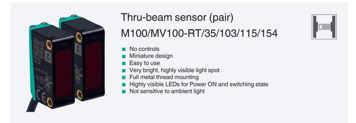
Thru-beam sensor, 20 m detection range, red light, dark on, DC version, PNP output, emitter switch-off, fixed cable
