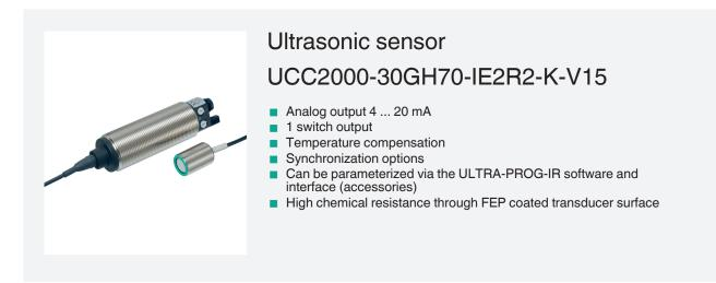
Ultrasonic diffuse sensor with separate transducer
