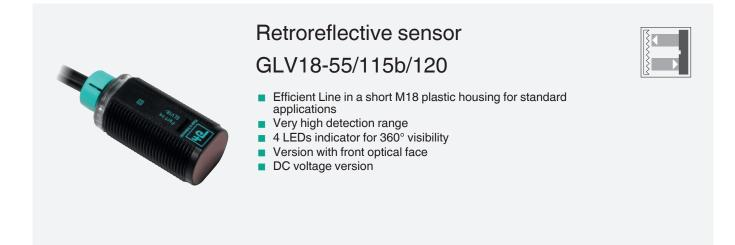
Retroreflective sensor with polarization filter, M18 threaded housing design, plastic housing, front optical face, 4 m detection range, red light, light/dark on, DC version, 2 PNP outputs, fixed cable with M12 plug
