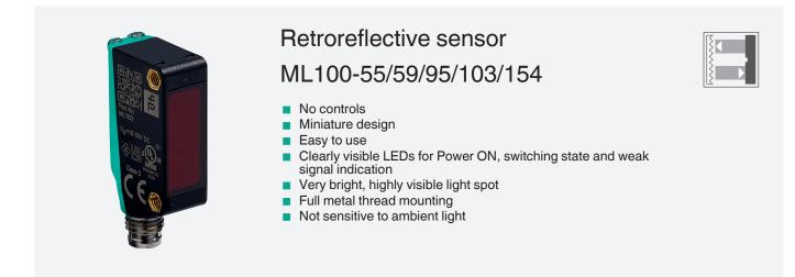
Retroreflective sensor with polarization filter, plastic housing, 5 m detection range, red light, dark on, DC version, PNP output, M8 plug
