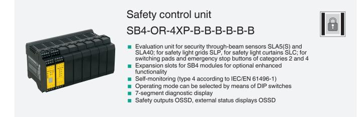
SB4 series safety control unit with optional module slots for functional enhancement
