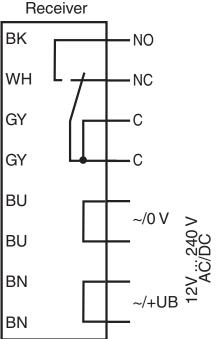
The relay-functions "NC" and "NO" bear on the switching mode "Dark-ON".
