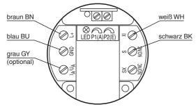
The terminals  $I_A/U_A$  (analog output) and SX ( $2^{nd}$  switching output) are not needed for programming.
