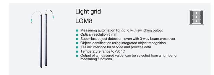
Measuring automation light grid with beam spacing of 8 mm, IO-Link interface, push-pull output, fixed cable with M12 plug
