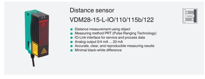
Universal distance sensor, measurement to object, IO-Link interface, measuring method: PRT, 15 m detection range, red laser light, laser class 2, push-pull output, analog output, fixed cable with M12 plug
