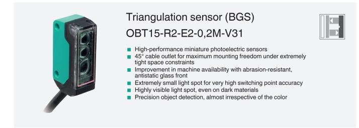
Triangulation sensor with background suppression for standard applications, miniature design, 15 mm detection range, red light, light on, PNP output, fixed cable
