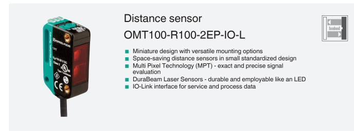
Measurement to object, 100 mm detection range, red laser light, laser class 1, measured value via IO-Link, 2 x push-pull output, 2 m fixed cable
