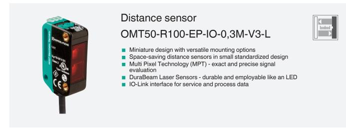
Measurement to object, 50 mm detection range, red laser light, laser class 1, measured value via IO-Link, push-pull output, fixed cable with M8 plug
