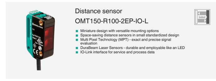
Measurement to object, 150 mm detection range, red laser light, laser class 1, measured value via IO-Link, 2 x push-pull output, 2 m fixed cable
