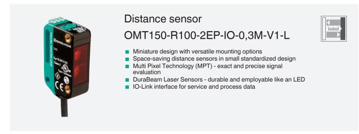
Measurement to object, 150 mm detection range, red laser light, laser class 1, measured value via IO-Link, 2 x push-pull output, fixed cable with M12 plug
