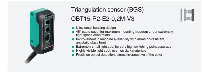
Triangulation sensor with background suppression for standard applications, miniature design, 15 mm detection range, red light, light on, PNP output, fixed cable with M8 plug
