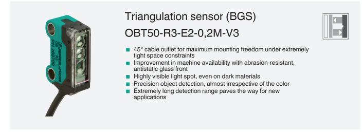
Triangulation sensor with background suppression for standard applications, miniature design, 50 mm detection range, red light, light on, PNP output, fixed cable with M8 plug
