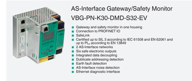
PROFINET Gateway with integrated safety monitor, double master for 2 AS-Interface networks, power supply input with decoupling coils
