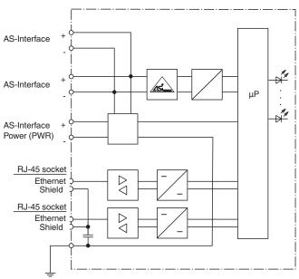
At the cable for power supply no slaves or repeaters may be attached.
