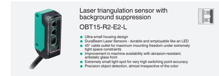
Laser triangulation sensor with background suppression, ultra-small design with M2 mounting, 15 mm sensing range, PNP output, 2 m fixed cable
