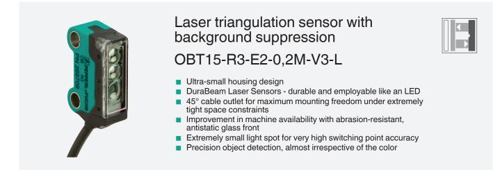
Laser triangulation sensor with background suppression, ultra-small design with M3 mounting, 15 mm sensing range, PNP output, 200 mm fixed cable with plug M8, 3-pin
