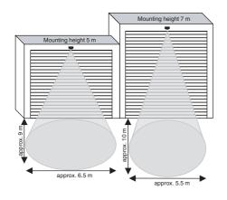
At maximum sensitivity and angle of incidence
