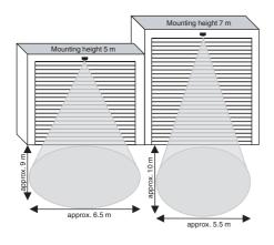
At maximum sensitivity and angle of incidence
