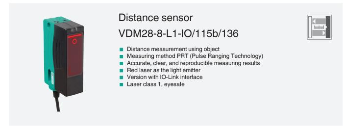
Universal distance sensor, measurement to object, IO-Link interface, measuring method PRT, 8 m detection range, red laser light, laser class 1, push-pull output, fixed cable with M12 plug
