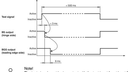
The test signal must be in contact with the test input for at least 9 ms! The duration of the test signal must not exceed 0.5 s, otherwise this will deactivate the sensor.
